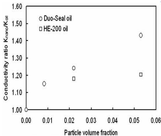
Figure 3. Conductivity Ratio of Nanofluid to Base Fluid versus Particle Volume Fraction [14]
