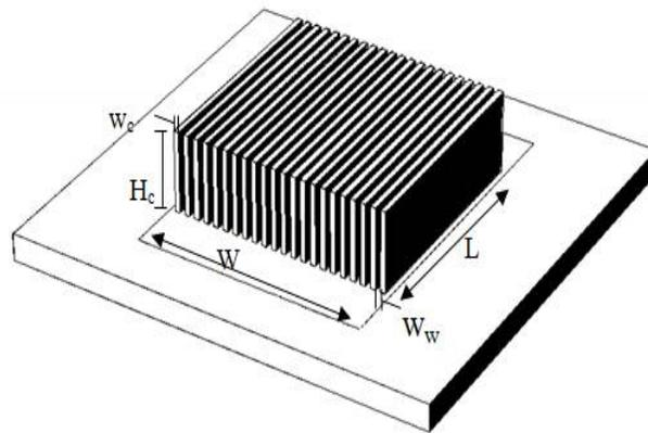
**Figure 1. Schematic of Microchannel Geometry for High Heat Flux Cooling Applications [19]**
