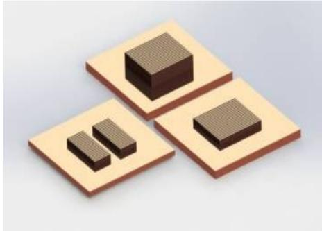
Figure 4. Double, Single and Split-Layered Microchannel [19]
