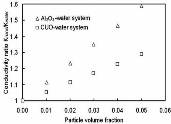
Figure 2. Conductivity Ratio of Nanofluid to Base Fluid versus Particle Volume Fraction [14]
